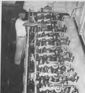
OILER F. R. Martina lubricates the valve lifters on the 12-cylinder diesel engine which will push the "Antilia" along at 12 to 15 knots.
